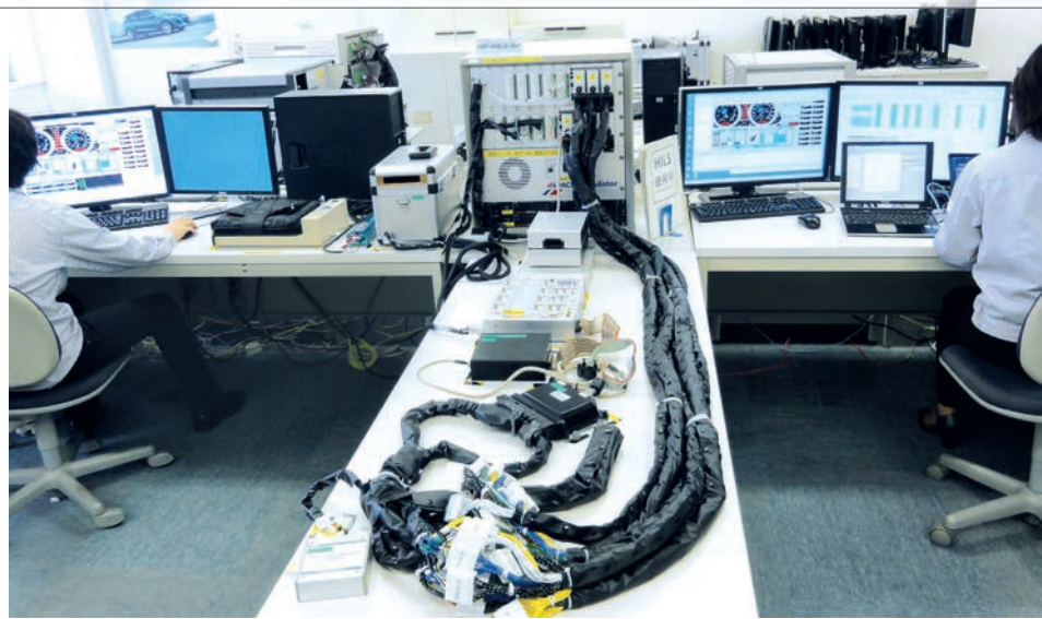
Figure 5: Test bench for the SKYACTIV-G ECUs.
